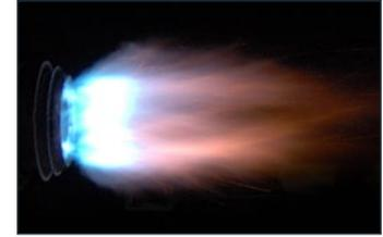
The compact flame shape eliminates drum overheating and does not require complicated flame shape adjustments for best combustion efficiency.
