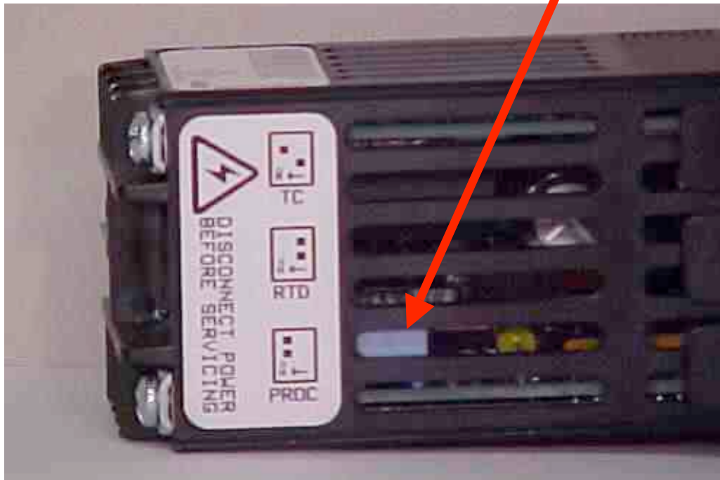
Figure 6: Input DIP Switches.
