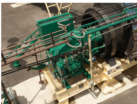
The Phoenix® Talon uses significantly less electric power than conventional burners due to the variable frequency drive used to control its combustion air blower and low body pressure.
