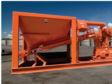
The coal prep skid pulverizes the coal for use by the burner.
