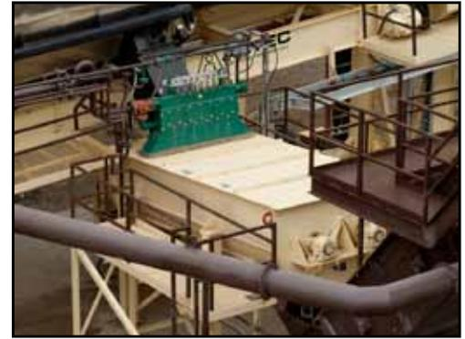
Virgin aggregate and RAP are discharged into a twin-shaft pugmill mixer/coater.
